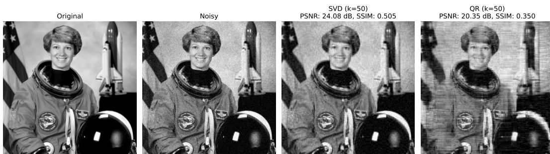
Fig. 9. Visual comparison at k = 50 . SVD preserves sharper edges; QR exhibits blur and structural loss.
