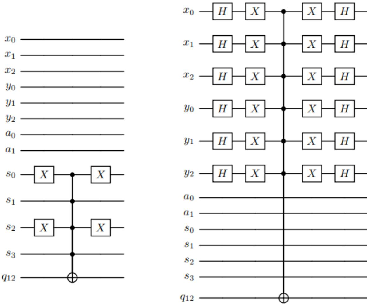
Fig. 2. Left: Diagram of the query circuit and its inverse used for the oracle operation,  $\mathcal{O}$ , for the case  $|s_0s_1s_2s_3\rangle = |0101\rangle$ . This circuit is run after the quantum adder circuit and is followed by the inverse quantum adder, forming a complete oracle. Right: The diffuser circuit used to amplify the solution(s).
