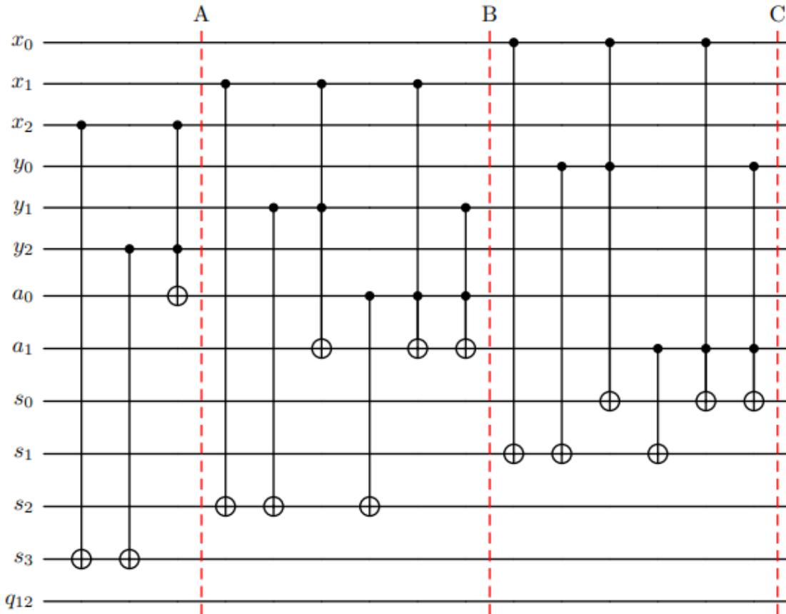
Fig. 1. A diagram of the quantum adder with barriers included to visually indicate each section.
