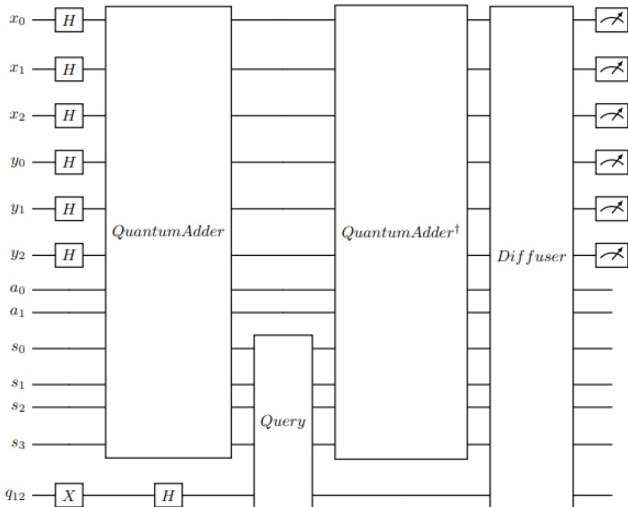
Fig. 3. The complete circuit employing one Grover iteration. The  $\dagger$  symbol indicates Hermitian conjugate.
