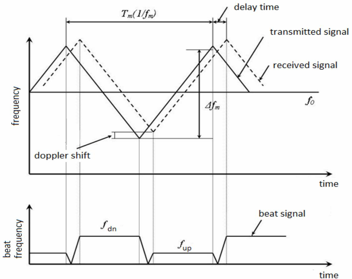
Fig. 1. FMCW triangular waveform and beating signal
