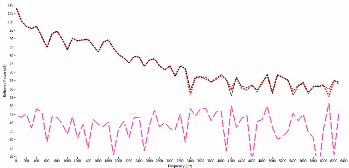
Fig. 6. Spectra of land clutter with a layer of 10 cm snow (solid – 1<sup>st</sup> period spectrum, points – 2<sup>nd</sup> period spectrum, dashed - difference)
