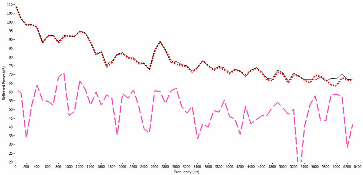
Fig. 5. Spectra of land clutter (solid – 1<sup>st</sup> period spectrum, points – 2<sup>nd</sup> period spectrum, dashed - difference)
