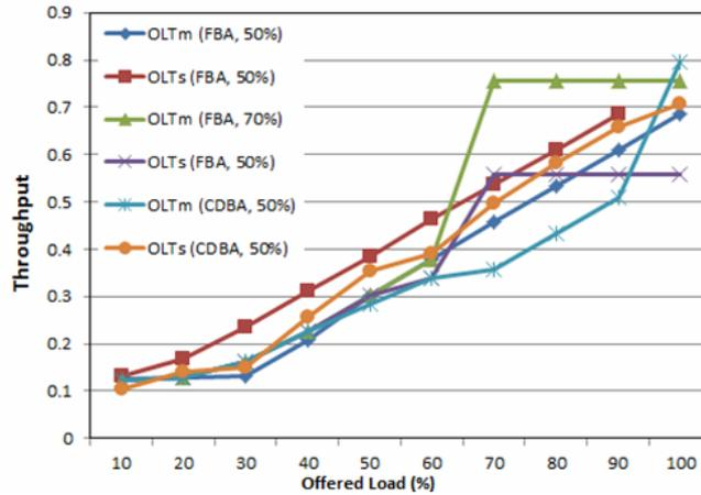
Fig. 6. Downstream throughput with assigned bandwidth ratio of 30%-70%.
