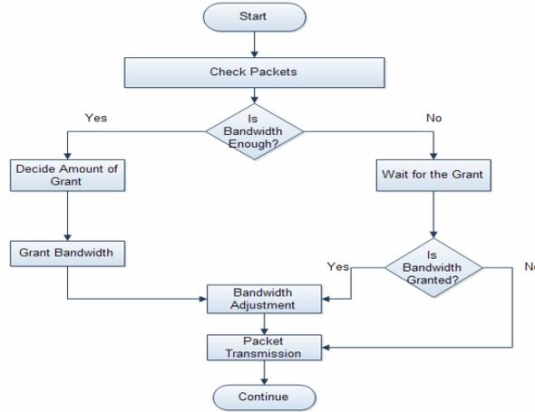
Fig. 4. Algorithm of Controlled DBA
