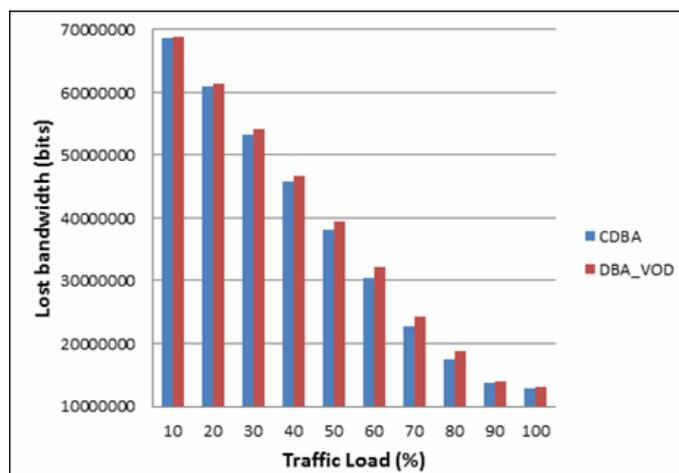
Fig. 7. Lost bandwidth ratio with traffic Load
