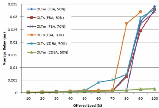
Fig. 5. Downstream delay with assigned bandwidth ratio of 30%-70%
