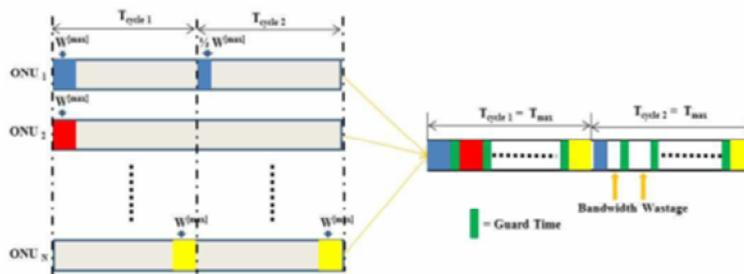
Fig. 2. Fixed Bandwidth Allocation Scheme
