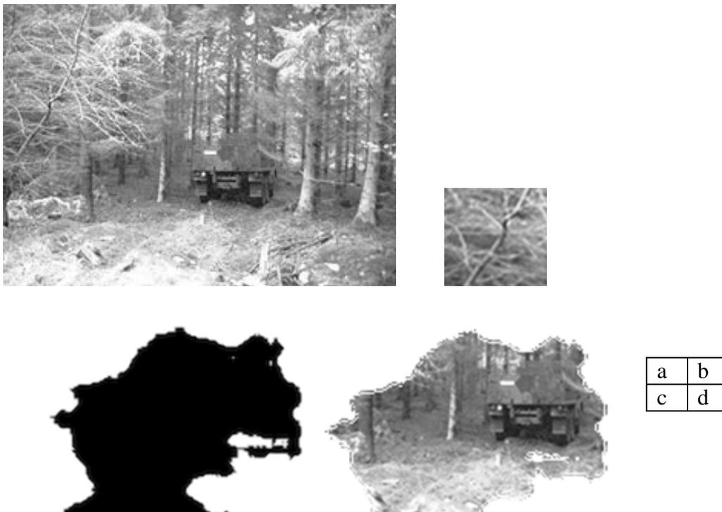
Fig. 1. Results of searching for detecting an anomaly. a- video frame with hidden object, b – image part without anomaly, c – binarized map of proximity measure, d – the part of whole image with minimal values of proximity measure.
