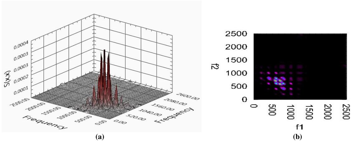
Fig. 4. Bispectrum estimation of the amount of carrier suppressed amplitude modulated and frequency modulated signals: default view (a) and top view (b).
