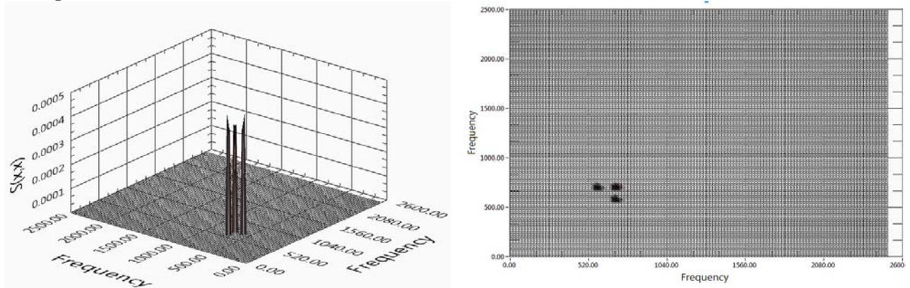
Fig. 6. Carrier suppressed amplitude modulated signal disclosing using bispectrum estimating.
