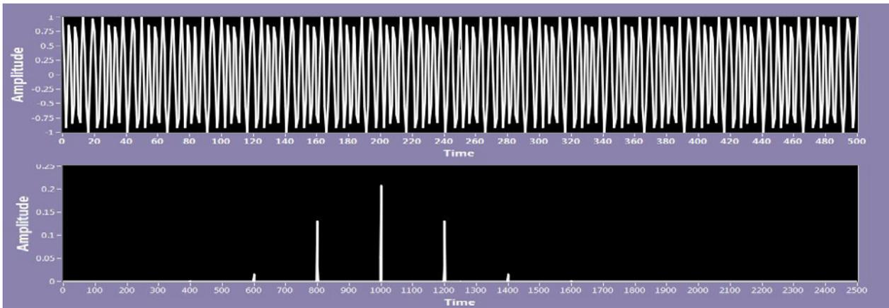
Fig.2. Time domain and power spectrum of frequency modulated signal.
