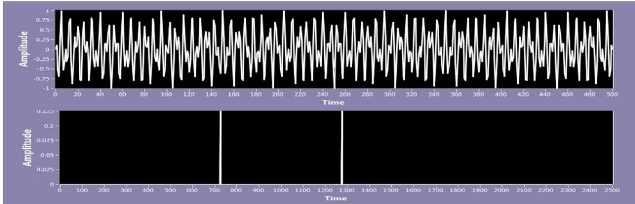
Fig.1. Time domain and power spectrum of carrier suppressed amplitude modulated signal.
