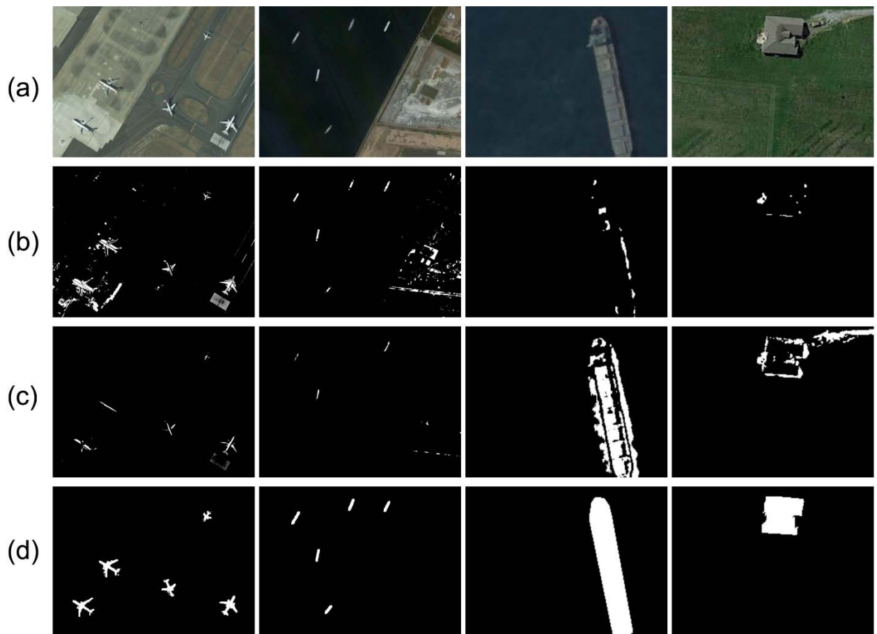
Fig. 4. Spectral residual saliency (SRS) detection: (a) input image, (b) output of SRS w/o enhancement, (c) output of SRS after enhancement, (d) ground-truth mask.
