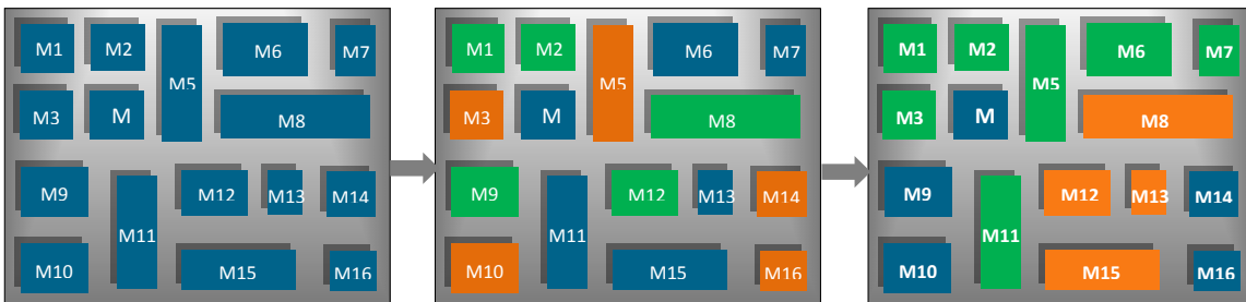
Fig. 1. Periodic test in the field: blue-colored blocks are in idle state, green-colored blocks are in mission and orange-colored blocks are in test mode.
