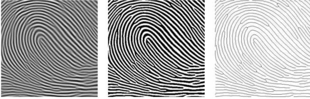
Fig. 1. From left to right: Original fingerprint image; Binarized image and the corresponding thinned image.
